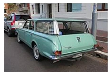
Image of an Australian built 1965 AP6 wagon with horizontal tail lamps, used on almost 60% of the build (6337 out of 10,853). This is very much like the 1965 Canadian base model Valiant 100 which had essentially the same front as the US model which used these tail lamps as well. These early Australian wagons used mostly imported panels such as doors, roof, quarter panels, tailgate, rear bumper etc. etc.
